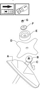
• Hook the blade guard/combination guard (A) onto the fitting on the shaft and secure with the bolt.
